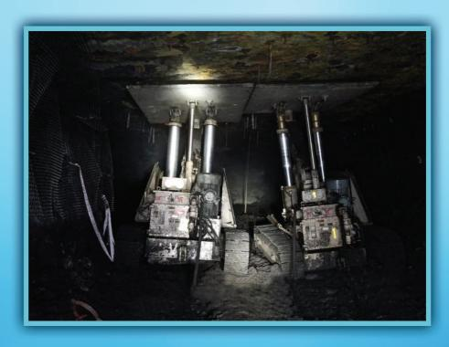
SELF ADVANCING (MOBILE) GOAF EDGE SUPPORT (SAGES) - 500 TONS CAPACITY FOR USE WITH CONTINUOUS MINERS
