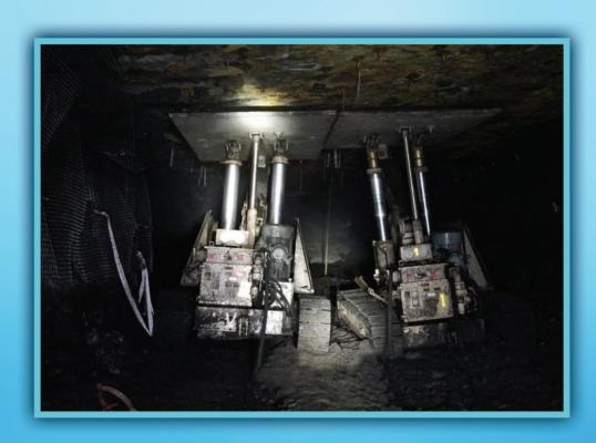
SELF ADVANCING (MOBILE) GOAF EDGE SUPPORT (SAGES) - 500 TONS CAPACITY FOR USE WITH CONTINUOUS MINERS
